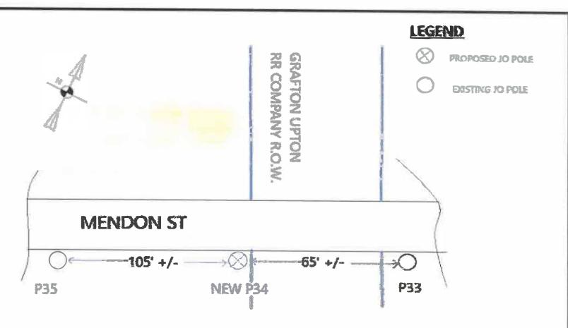
National Grid respectfully request permission to install new intermediate pole 34 Mendon St for purpose of raising existing facilities for new Railroad Signal Gate
